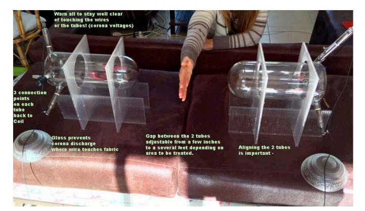
Use caution when connecting and operating the device. The input side of the Tesla resonator is the connection to a high voltage transformer and carries a high current load. Contact with the input terminals of the large box containing the Tesla resonator or the output leads of the amplifier while in operation will result in a potentially lethal shock. Always make sure the device is unplugged from the mains while connecting the Tesla resonator and plasma tubes.
