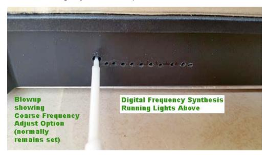
To adjust the coarse tuning locate the coarse tuning hole to the left of the LEDs on the front face of the amplifier. Use the included small flat head adjustment tool to adjust the small potentiometer inside the amplifier next to the green LEDs. It is a small brass flat head screw on a blue rectangular base.
