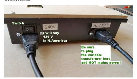
Make sure the amplifier power switch is in the off position and the main input power cables are disconnected from the wall while setting up the apparatus.
